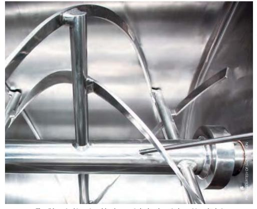
The ribbons in this sanitary blender are pitched and precisely positioned relative to one another to generate vigorous flow, both radially and axially.
