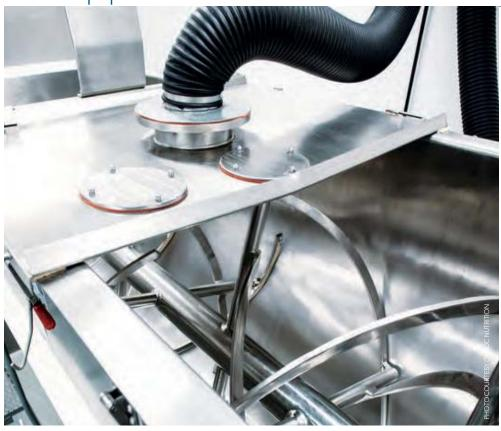
The quick discharge, easy cleaning, and low risk of cross-contamination facilitated by a sanitary design and finish are especially important for a high-volume contract manufacturer. This blender is also equipped with dust collection to promote a clean working environment for the manufacturing team.
